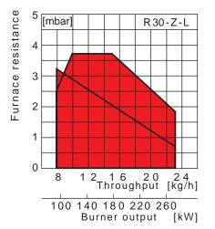
working ranges tested in accordance with DIN EN 267
