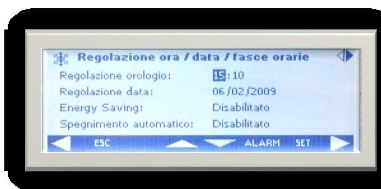
If the Energy Saving mode is enabled during specific time slots, the controller will adapt the set point values dragging them to modifiable values.
