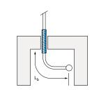
If the shaft is too small to fit the calculated expansion bend, the hole in the wall will have to be made larger to give the pipe sufficient room for movement. The pipe must be provided at the hole in the wall with PE insulation.
