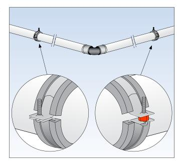
The correct placing of sliding points and fixed points is very important when expansion bends and expansion loops are used. Expansion bends must be fitted if the pipe changes direction.
