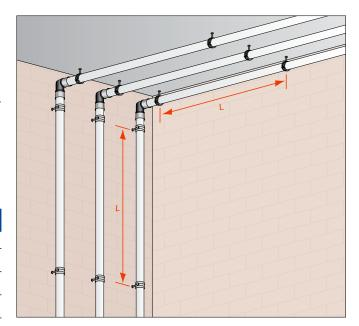
The **pipe brackets** have a twofold purpose; firstly they support the pipe network, and secondly they accommodate the thermal length changes of the pipe with **sliding and fixed points**, usually in combination with correctly calculated expansion bends and expansion loops. The sliding points must be such that the pipe continuously has clearance. The sliding point may not become a fixed point when the pipe expands.
