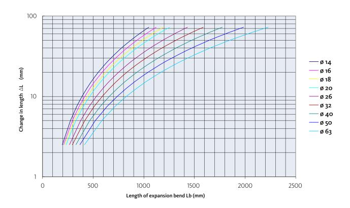
It must also be ensured that pipes can freely move **when piping runs from floors to a riser pipe in a shaft**. Also here, the change in length can be accommodated by an expansion bend. The expansion bend will then accommodate the upward and downward movements.
